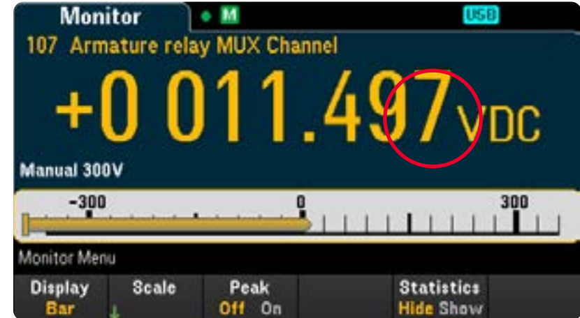
Figure 17b. Lowest voltage resolution (sensitivity) at 300 V range
